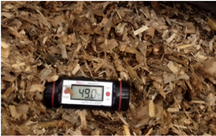
Figure 1: Spear-thermometer indicating 49°C at the cutting edge of a corn silage with ambient temperature of 18°C.
